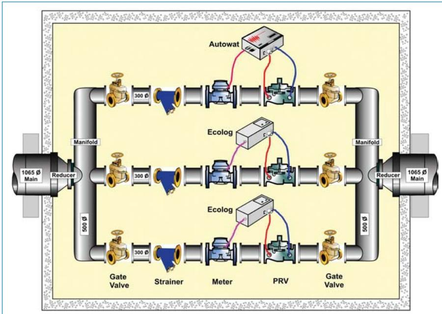
**Figure 2.** Schematic Layout of the 1065 mm diameter Installation.
