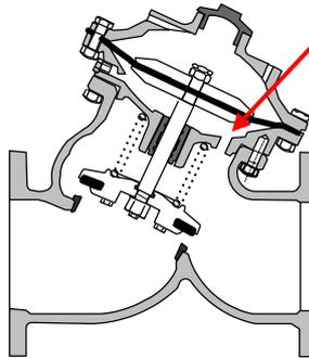
"Y" type valve, converted to single chamber design by opening bores in the bottom chamber
