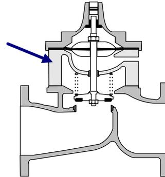
Typical conversion to double chamber in common globe type valves
