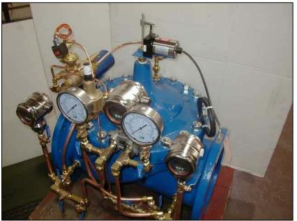
Figure 2 - Cla-Val Flow Modulated PRV Assembly
