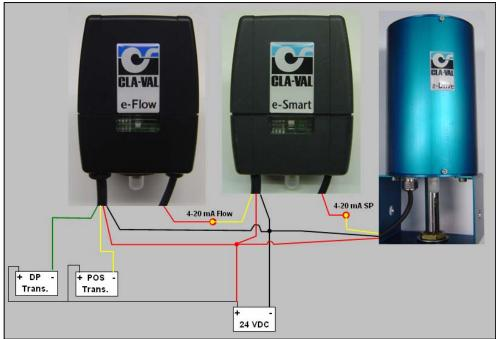
Figure 3 - Cla-Val Flow Modulation Controller Wiring
