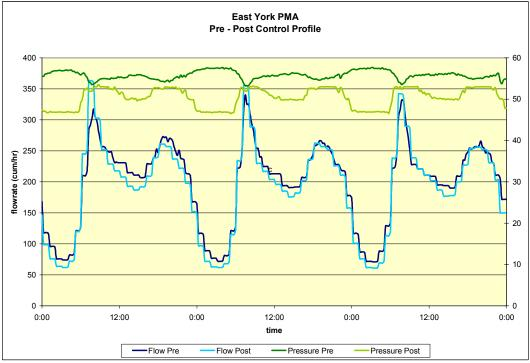
Figure 7 - No-Control vs. Control PMA Flow & Pressure Profile
