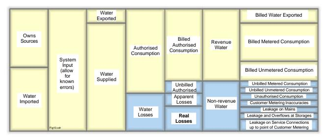
Figure 5: Main components of the water supply water balance
