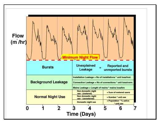
Figure 4: Components making up the minimum night-flow
