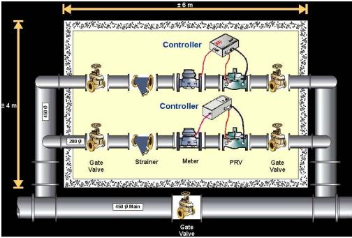
Figure 3 Schematic layout of the 450 mm diameter installation
