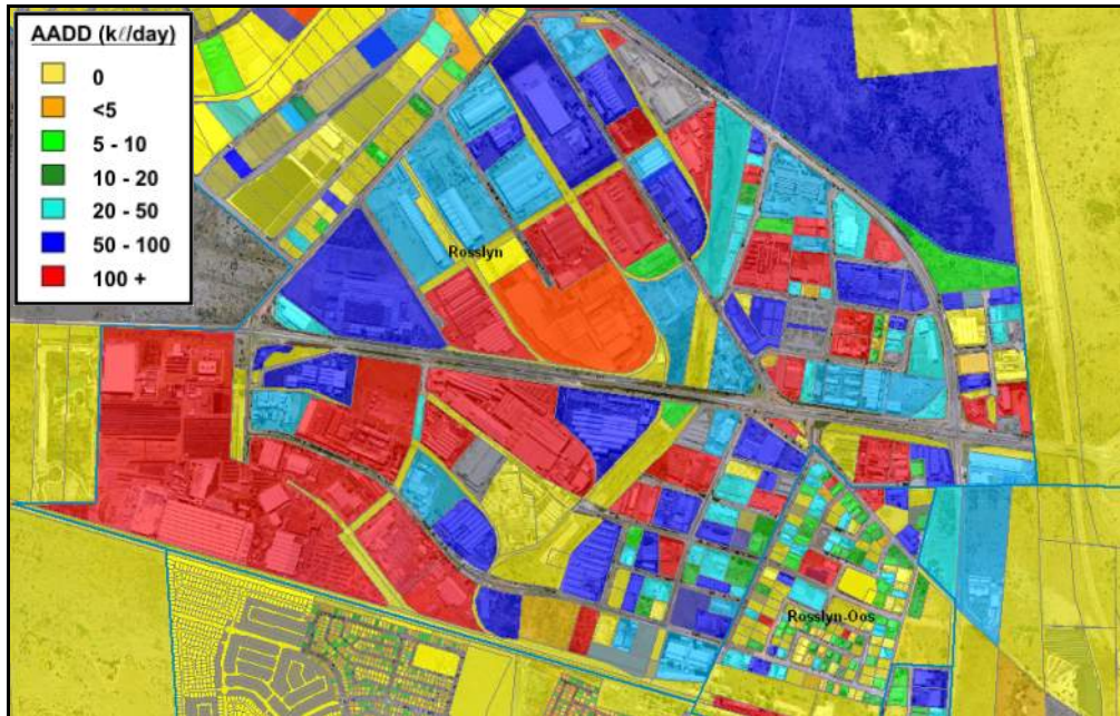
Figure 3: Screen from Management Information System of the City of Tshwane showing the Average Annual Daily Demand (AADD) for the different stands in an industrial area.
