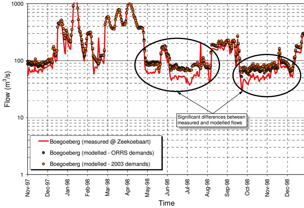
Figure 3: Measured flows versus modelled flows at Boegoeberg (1998)
