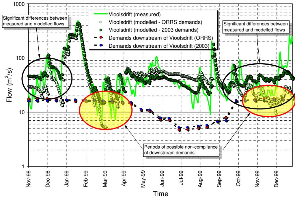
Figure 6: Measured flows versus modelled flows at Violsdrift (1999)
