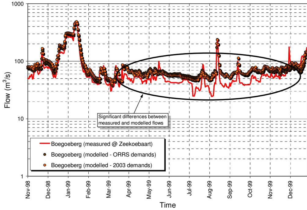
Figure 5: Measured flows versus modelled flows at Boegoeberg (1999)
