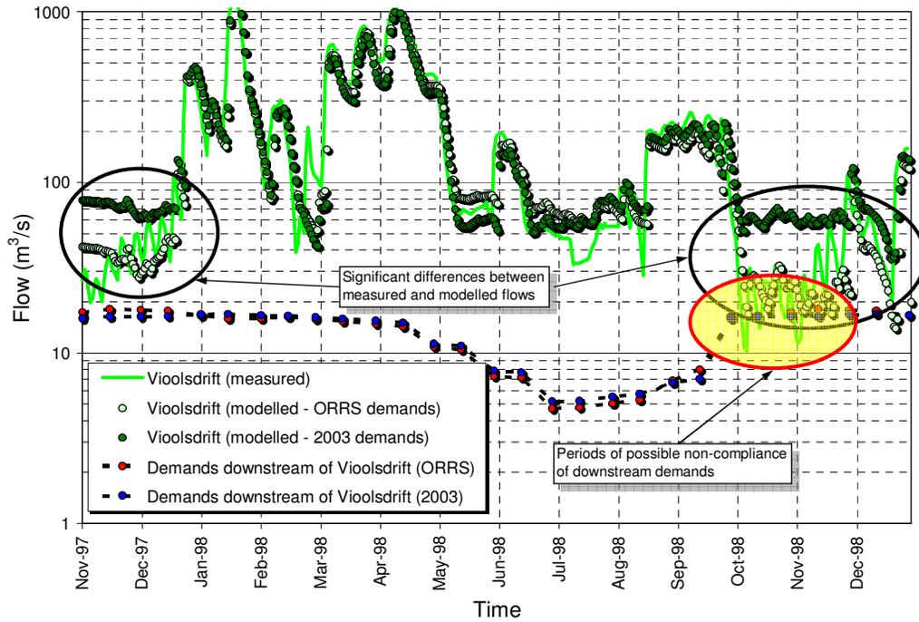
Figure 4: Measured flows versus modelled flows at Violsdrift (1998)
