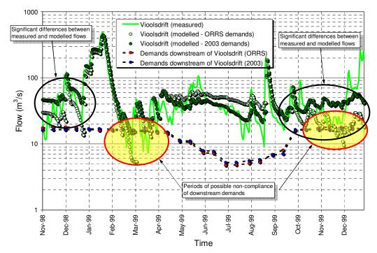
Figure 6: Measured flows versus modelled flows at Vioolsdrift (1999)
