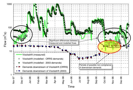
Figure 4: Measured flows versus modelled flows at Vioolsdrift (1998)
