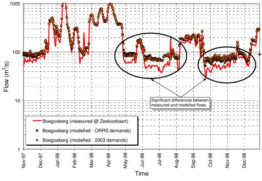
Figure 3: Measured flows versus modelled flows at Boegoeberg (1998)
