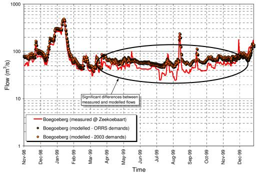
Figure 5: Measured flows versus modelled flows at Boegoeberg (1999)
