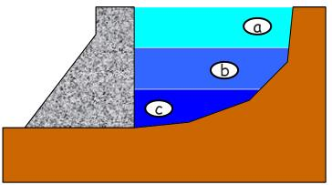
Figure 8: Section through re-regulating dam showing different theoretical storages
