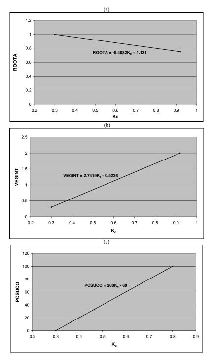
Figure 2.1. Linear relationships between (a) ROOTA and K<sub>c</sub>, (b) VEGINT and K<sub>c</sub> and (c) PCSUCO and K<sub>c</sub>
