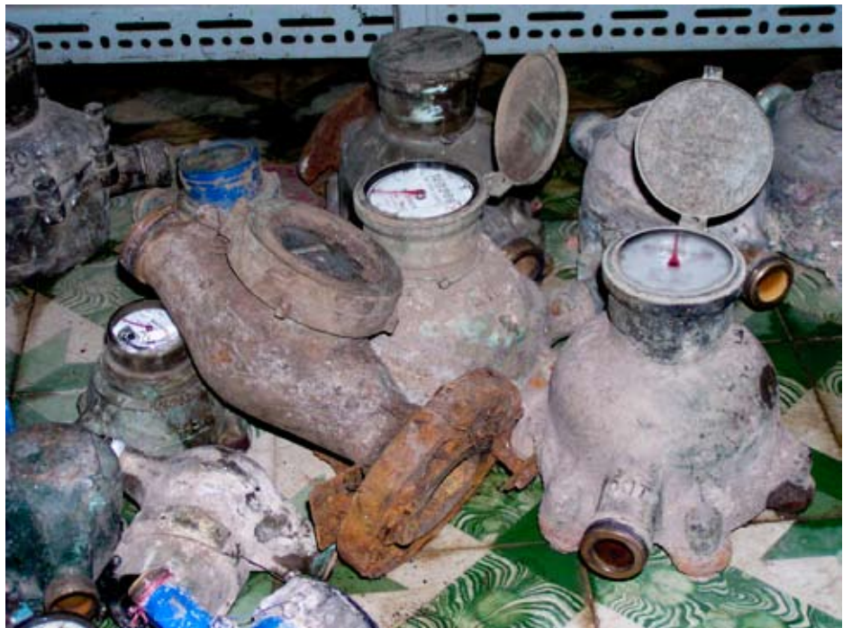
Deteriorated customer meters
